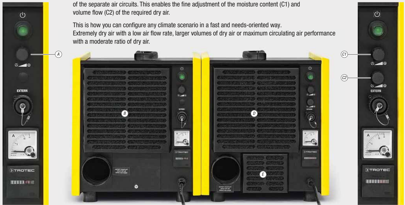
The model differences at a glance: On the left: a TTR 400 with Monoventic air volume regulation (A) and a common inlet for both air flows (B); on the right: a TTR 400 D with Duoventic regulation (C1, C2) and separate inlets for dry air (D) and regeneration air (E).
